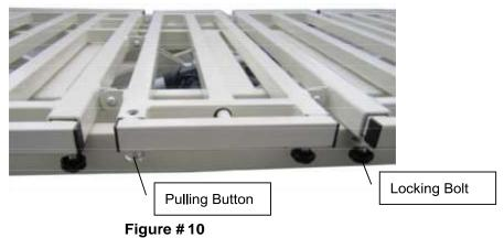
4.2 **IMPORTANT NOTE:** There are 3 location holes on each extension frame for 3 width adjustment settings - 36", 42" and 48" widths. There are 4 separate extension frames on each side of the main frame. Repeat the above method in 6.1 to achieve the desired width and then tighten the "Locking Bolt" to lock the extension frame in place. See Figure # 10A.
