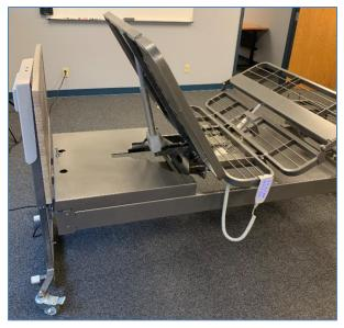
2. Locate and remove the two bolts pictured below that hold the actuator into place. Once removed, install the actuator to the corresponding holes on the opposite side of the bed.
