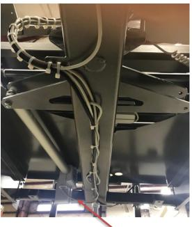
Actuator mounted in "Left turn Position"
