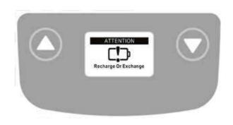
If the battery is critically low, the LCD Display Panel will show the sign on the left either when the emergency stop button is released or when a button on the LCD Display Panel is pressed.
