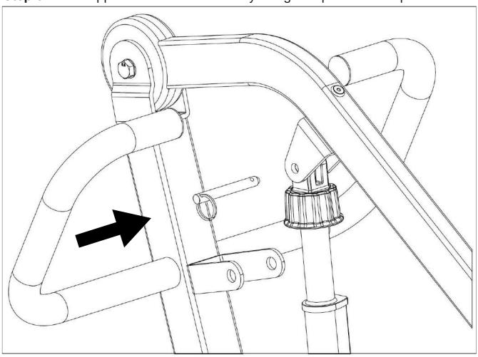
**Step 7**: Install spreader bar into the boom as shown.
