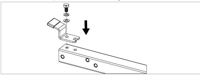
**Step 3**: Lock the rear casters on the base and insert the mast into the base bracket by aligning the holes. Secure the mast to the base using the hardware as shown. Use wrenches to tighten the hardware.
