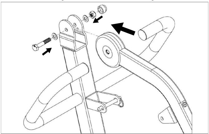
**Step 5**: Move the boom out of the way and install lower end of actuator as shown. It is critical to have motor part of the actuator face the same direction as the big arrow.
