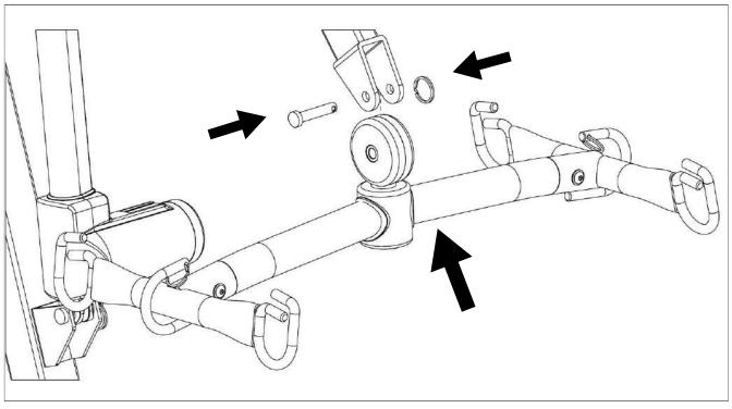
**Step 10**: Install the control unit to the frame as shown.
