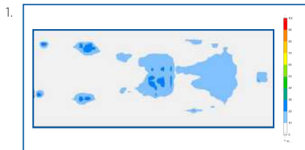
1. Test shows subject in supine position demonstrating contact measurement between key pressure points using Boditrak mapping technology on the SPS1084 support surface. Subject: Male 5'11", 185 lb.
