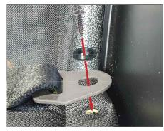
With the top of the belt facing up, place the washer over the seat belt hole. Thread the screw through the washer and the hole in the belt and line it up with the hole in the seat.
