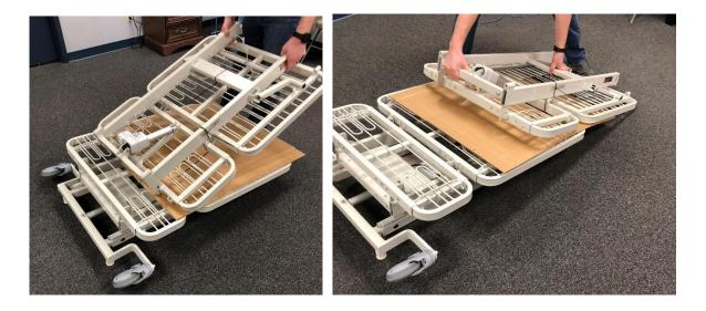
7. Unbolt the other two 7/16-14" X 4 ½" Bolts and remove the head section assembly from the head high low assembly. Remove and retain hardware for assembly process.
