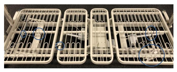
9. Plug the high low cable into actuators, use the provided c-clips to secure the cable (be sure to push in until flush with plastic housing). Route the wire along the weldment and secure with the provided cable ties. Cut off any excess cable tie.
