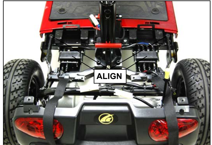
FIGURE 21. CORRECT FRAME ALIGNMENT
