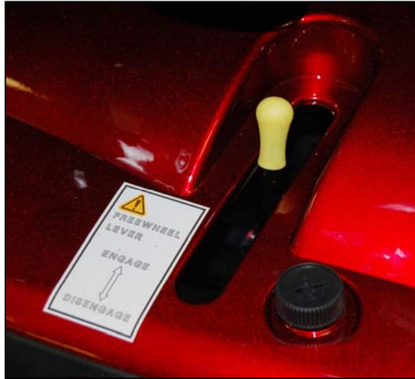
FIGURE 11. FREEWHEEL LEVER (ENGAGED)
