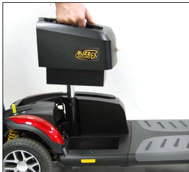
Figure 21. Battery Pack Installation
